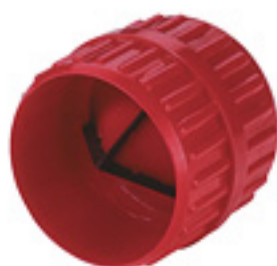
>>> CT-208 Inner-outer reamer (Plastic body) Reaming capacity~3/16" to 1-1/2" O.D. (1/8"~1-1/4" nom)
